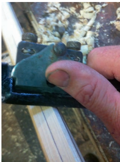
A spoke shave can also be used to remove the arras. Use your block plane first though..
