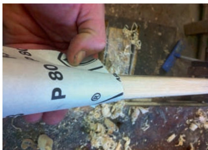
Use 60 or 80 grit paper in a wrap-around method to smooth the arras further.
