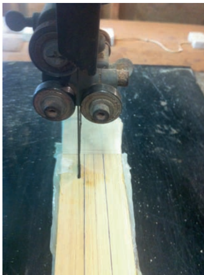
Cutting out to the lines, leave around 1/8in on.
