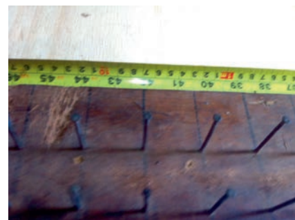
Clamp your jig at the correct length in line with the jig's side mark.
