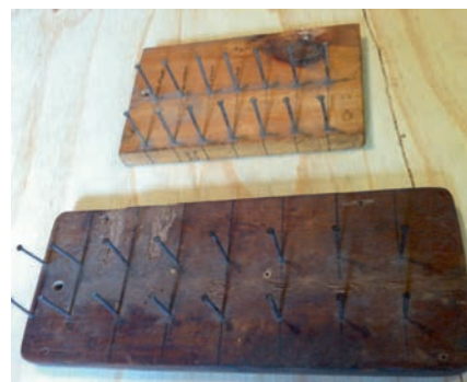
Two- and three-bundle jigs. The bottom one is the three-bundle jig. Note how spaced out the nails are.
