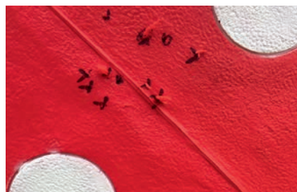
The back: Of the 150 arrows shot at the block, only 11 made it to the opposite side (highlighted with a marker).
