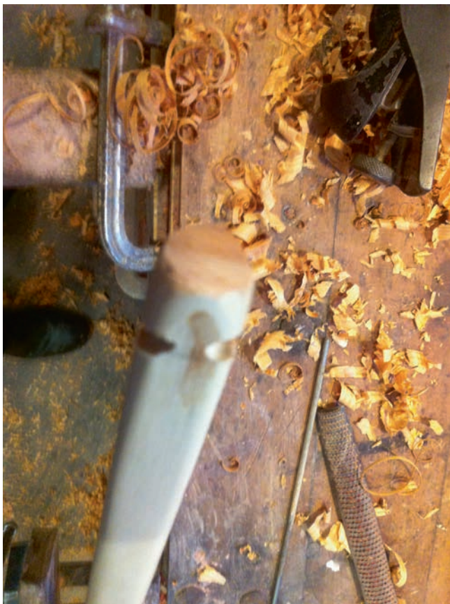
Perfect tillering nock alignment is critical.
