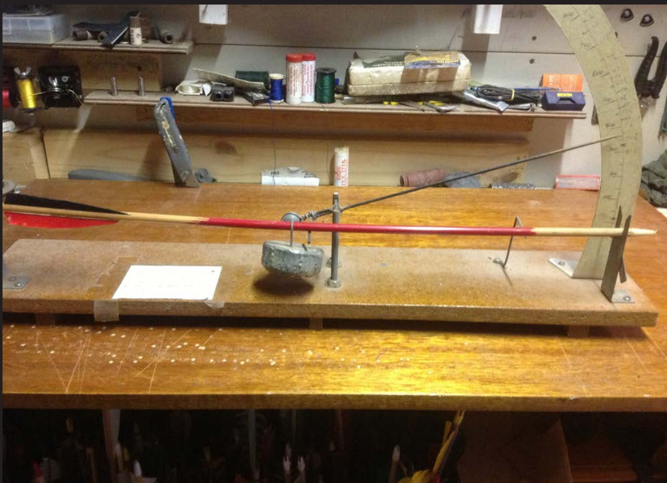
Basic static spine testing. 2lb weight suspended from the shaft's centre on a 26 inch span
